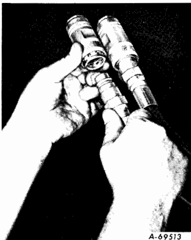
Illustr. 30A Connecting the self-sealing couplings on the side mounted junction blocks.
