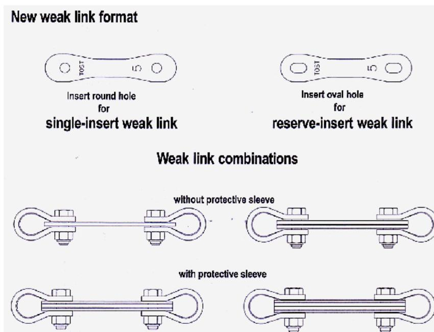
TOST weak links are color coded for easy selection and verification. TOST specification for these links are shown in the following chart. The choice for each CSA sailplane is shown in the right column.
